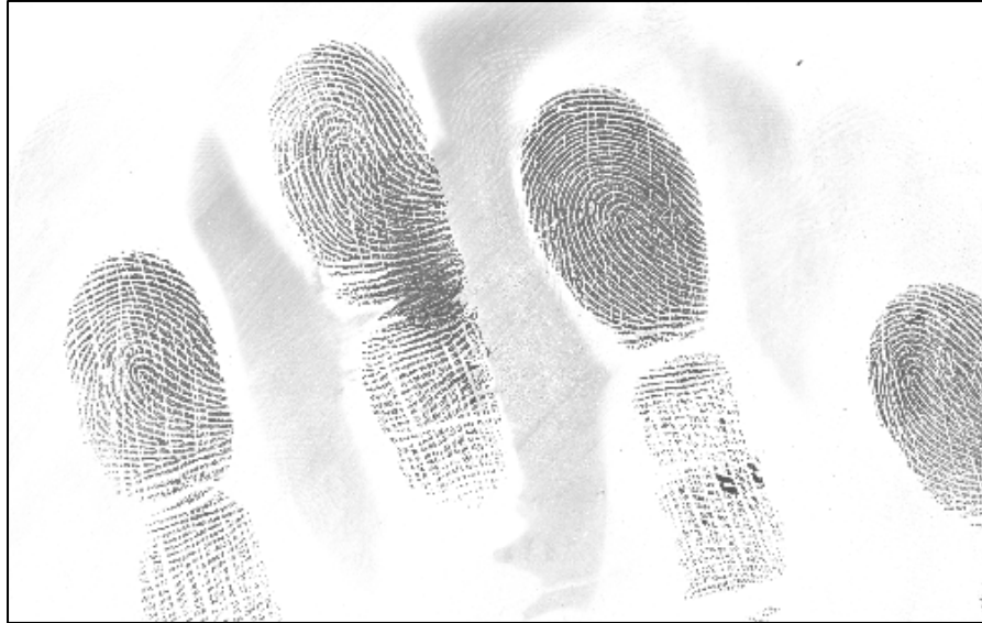
Figure 4. Moisture/Condensation on the platen surface.
