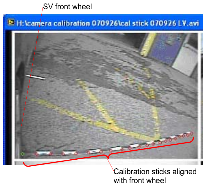
Figure 6. Calibration of side camera using meter sticks.
