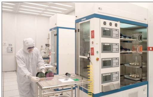
Figure 2. Oxidation and annealing furnace banks.
