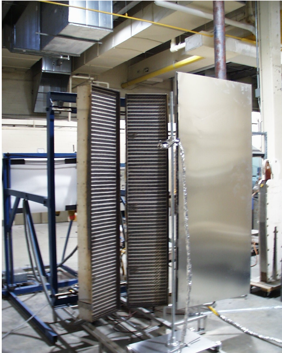
Figure 5. Photograph of radiant panels and radiation shield with trolley mounted heat flux gauge.
