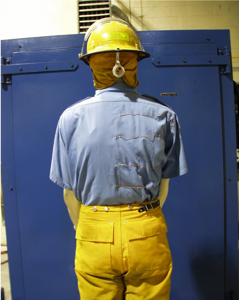
Figure 11. Photograph showing mannequin without coat and instrumentation (heat flux gauge and thermocouples).
