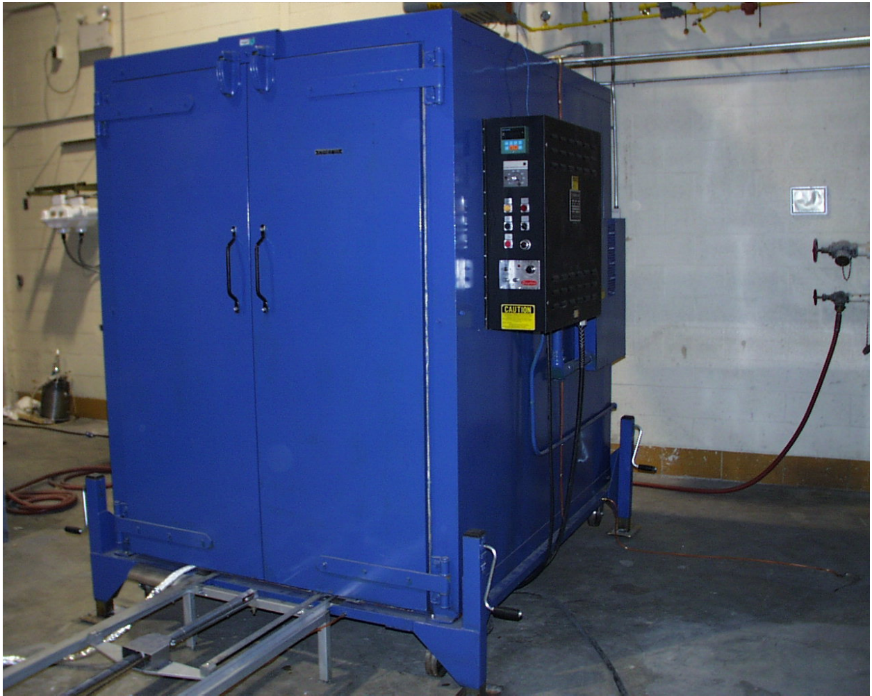
Figure 6. Photograph of the preconditioning chamber.
