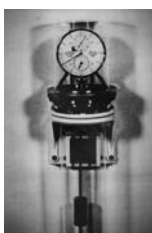
NBS Pendulum clock (1904) 1s in 3 years
