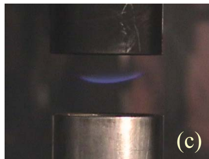
Figure 9. Photos of extinction process of a 1-g counterflow nonpremixed flame for a_g=20 \text{ s}^{-1} and Vr=3 , with Ca increasing from 0.79 to 0.825.
