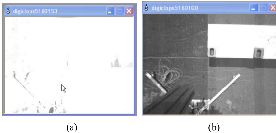
Figure 8 Stereo Camera in Sunlight, (a) without filter (b) with filter
