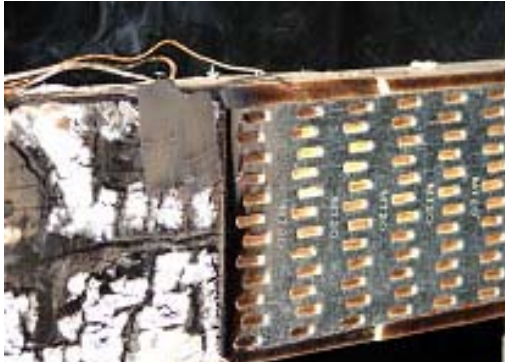
Figure 11 - 10 minutes into the test the plate is still shiny
