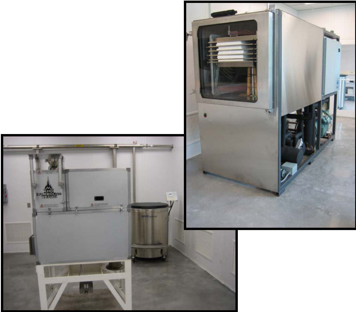
Figure 7. Vibrating Cryomill (left) and Freeze-Dryer (right) Located in the Reference Materials Production Facility
