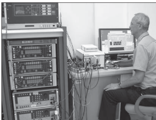
PMUs – a key component of electric power grid modernization. The figure shows the NIST Calibration System for PMUs. The PMUs are the two instruments on top of the cabinet.
