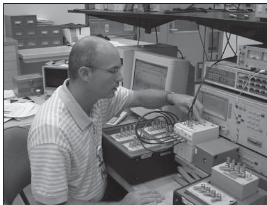
Andrew Koffman performs a special test for a four-terminal-pair capacitance standard.
