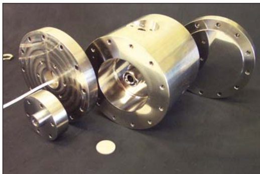
Figure 2. Second-generation acoustic viscometer made from Monel for use with corrosive gases.
