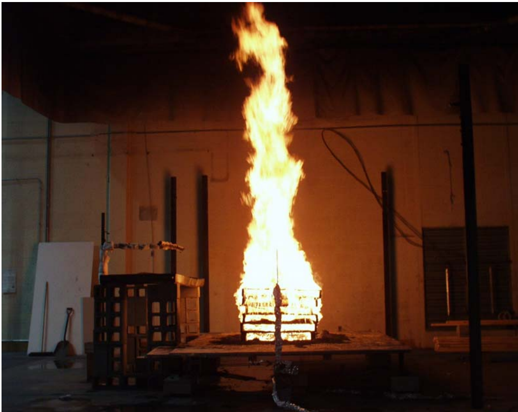
Figure 16. Pallet Test at Maximum Heat Release Rate
