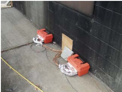
Figure 34. Pressure Transducer Implementation
