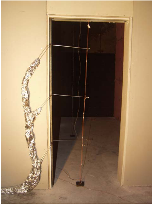
Figure 12. Doorway and Passageway Instrumentation and High Temperature Panels
