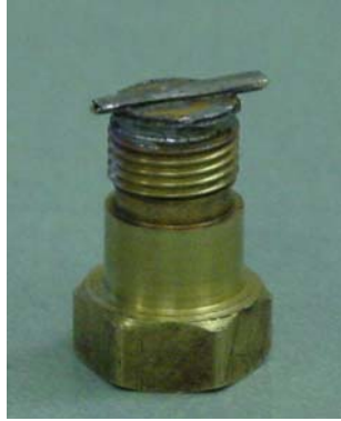
Figure 6.19 Oil Capsule Top Connected to Flow Restrictor
