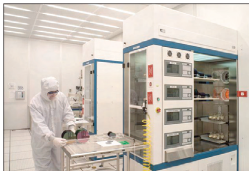
Figure 2. Oxidation and annealing furnaces banks.
