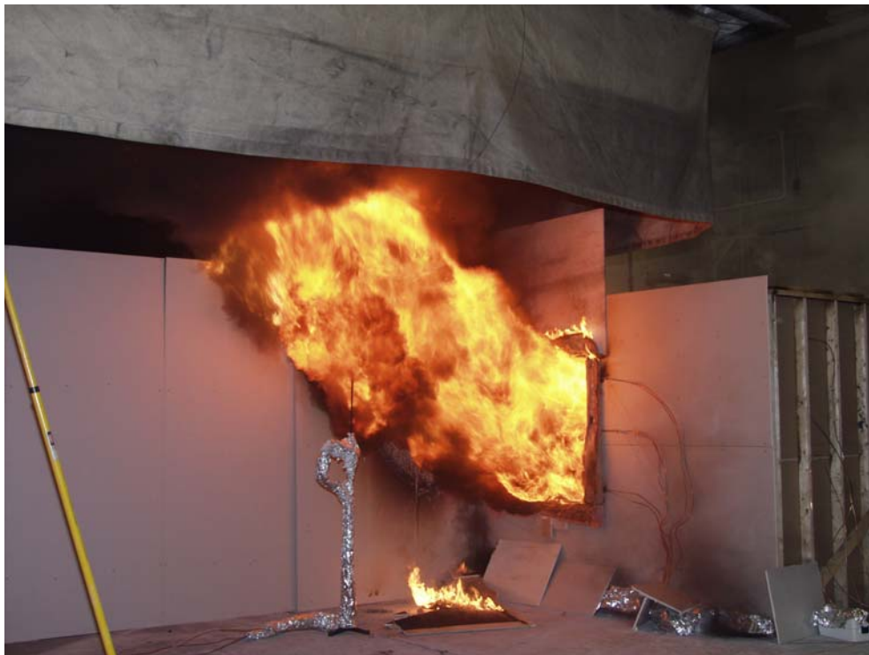
Figure 4-23. Exterior View of Window After the Start of Forced Ventilation (380 s)
