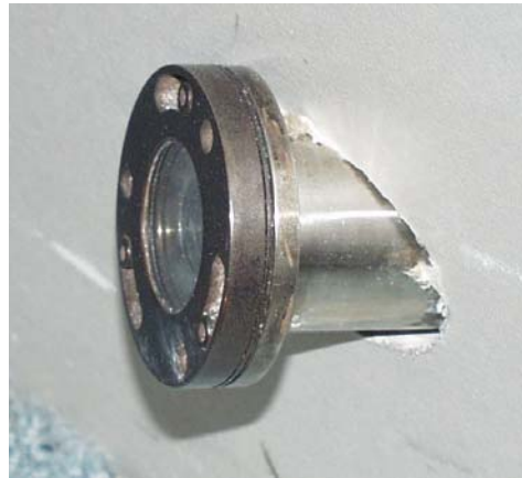
Figure 4-9. Water Cooled Camera
