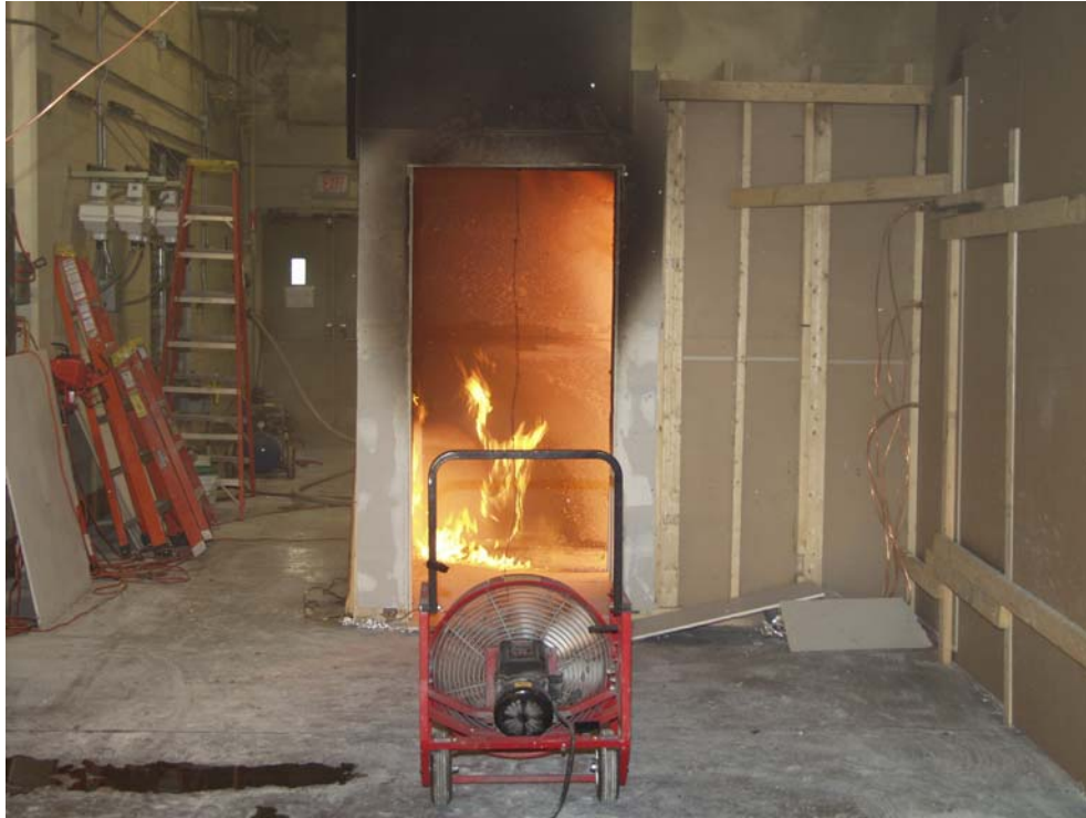
Figure 4-22. Exterior View of Doorway to Corridor After the Start of Forced Ventilation (470 s)
