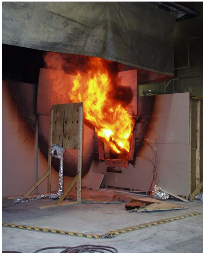
Figure 4-25. Window During Natural Ventilation Experiment (470 s)
