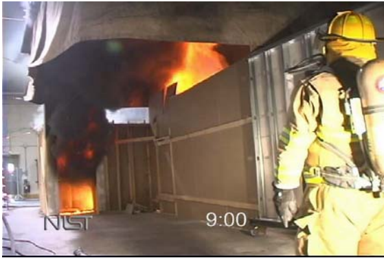
Figure 4-58. Fire in Decay Stage (540 s)
