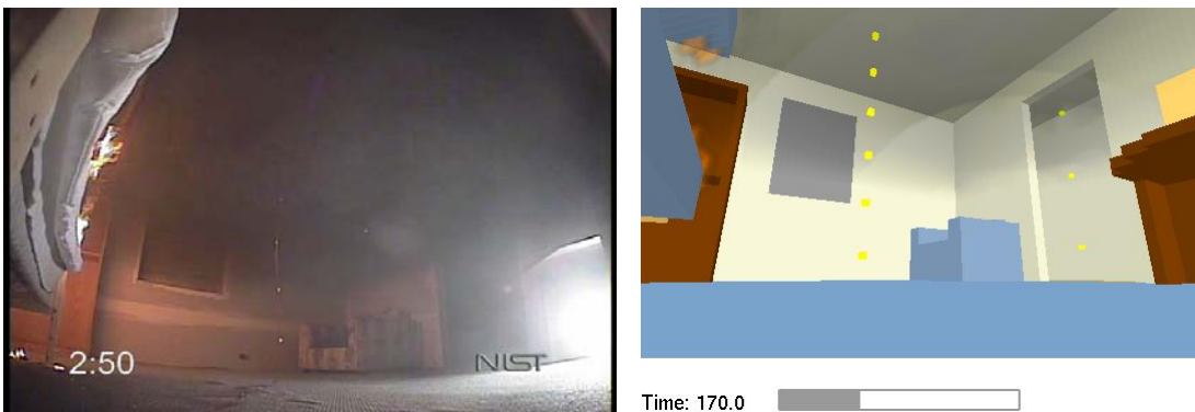
Figure 4-69. Doorway and Window View as Flames Spread to Top Mattress (170 s)
