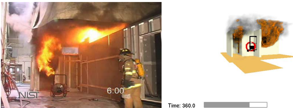
Figure 4-74. Doorway View 10 s After Fan is Turned On (360 s)
