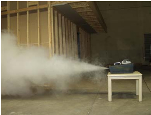
Figure 2-8. Smoke Generator Flowing
