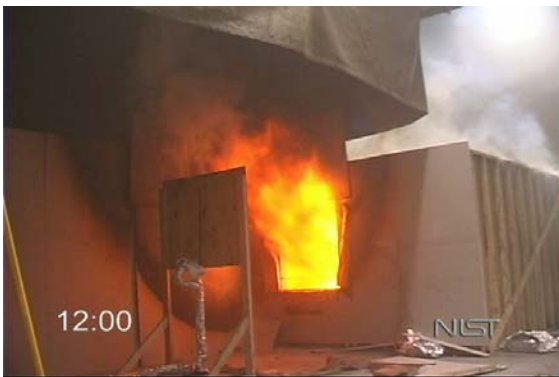
Figure 4-59. Room Continues to Burn (720 s)
