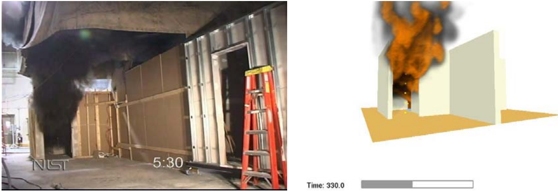
Figure 4-54. Combustion Products Flow From Corridor Doorway (330 s)
