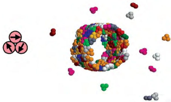
Figure 2: Tubular structures (right) arise from the simulated organization of triangular arrangements of dipole particles, shown schematically at left.
