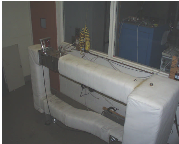
Figure 6. Photograph of flow loop experimental apparatus.
