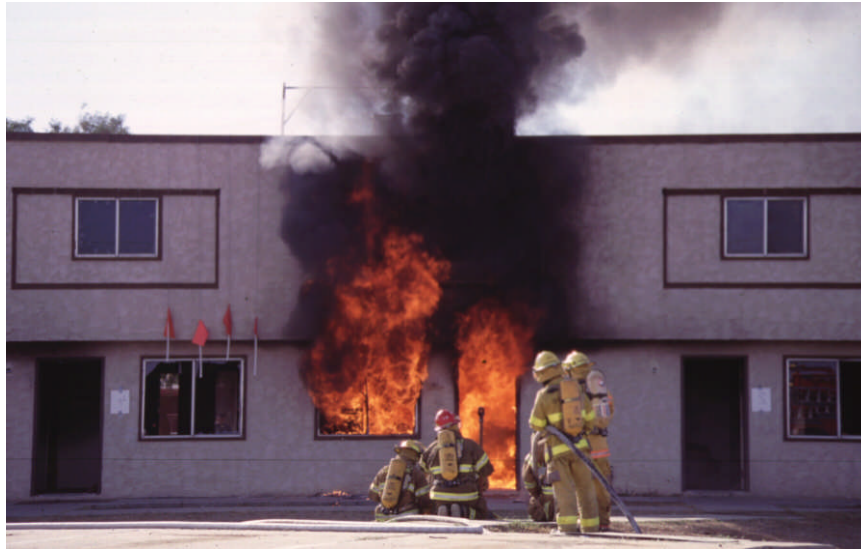
Figure 11. Full-scale townhouse fire test used to expose instrumented mannequin.
