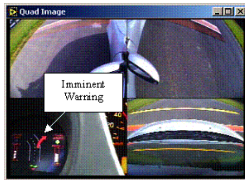
Figure 5. Curve speed imminent warning indicated by long arrow.
