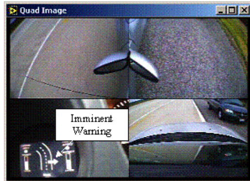
Figure 3. Lateral drift imminent warning indicated by arrow at 3 o'clock.
