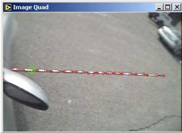
Figure 17. Red circles show pixels corresponding to segments on cal stick. Use the “Move Reference Points” control panel to adjust circle locations. Green circle is one being moved after setting “Point #” to 3 (see Figure 16).
