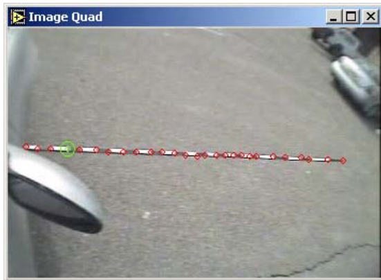
Figure 7. Calibration sticks for side view camera.
