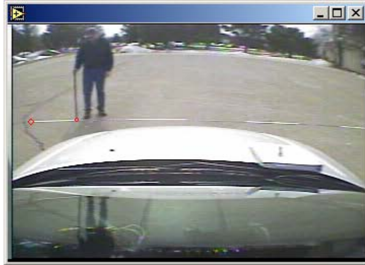
Figure 18. A user pointing to the control points using a colored meter stick.
