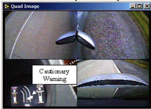
Figure 2. Lateral drift cautionary warning indicated by arrow at 2 o'clock.
