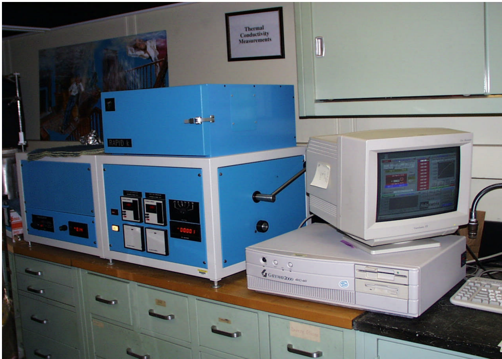
Figure 1 Rapid-k thermal conductivity test apparatus and computer system.
