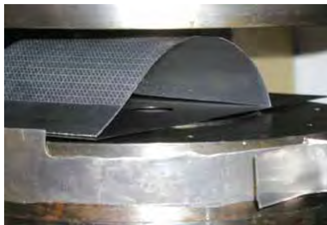
Figure 1: NUMISHEET benchmark sample loaded for plane strain deformation.
