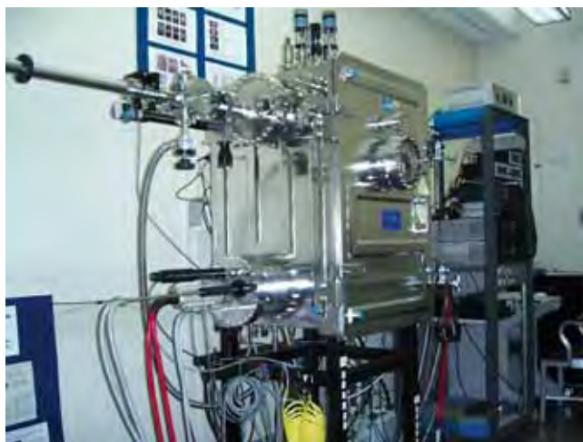
Figure 10: The combinatorial thin-film deposition system has a base vacuum in the low 10^{-8} Torr ( 10^{-6} Pa) range and is equipped with a load-lock for specimen transfer.
