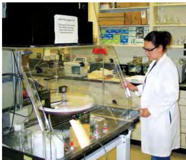
Figure 17: Yamali Hernandez keeps a watchful eye on the Langmuir-Blodgett trough in one of the NCNR's recently renovated user laboratories.
