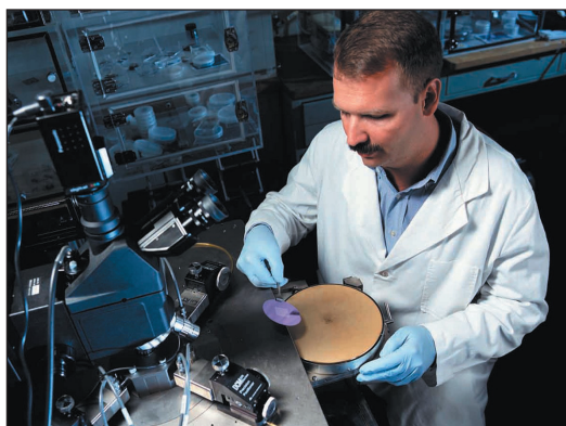
Figure 1. Curt Richter loads a molecular electronic sample for electrical characterization.
