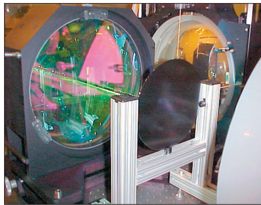
Figure 1b. Test end of the IR 2 setup for TTV measurements of 300 mm wafers. The picture shows the collimator lens together with a silicon wafer and a return flat.
