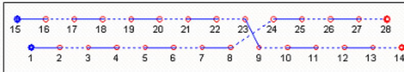
Coil Circuitry (right slab as seen below)
