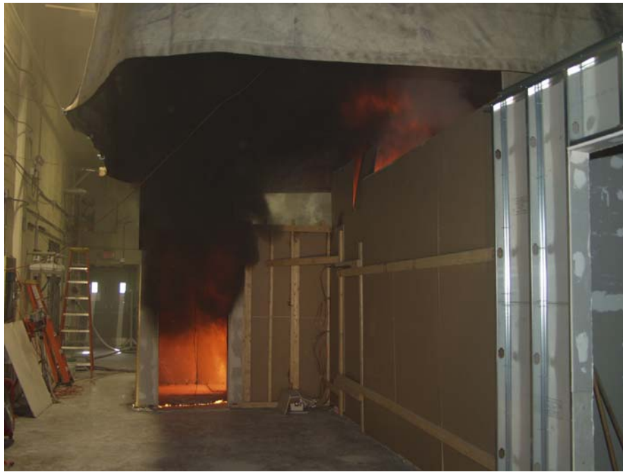
Figure 26 – Doorway During Natural Ventilation Experiment (645 s)
