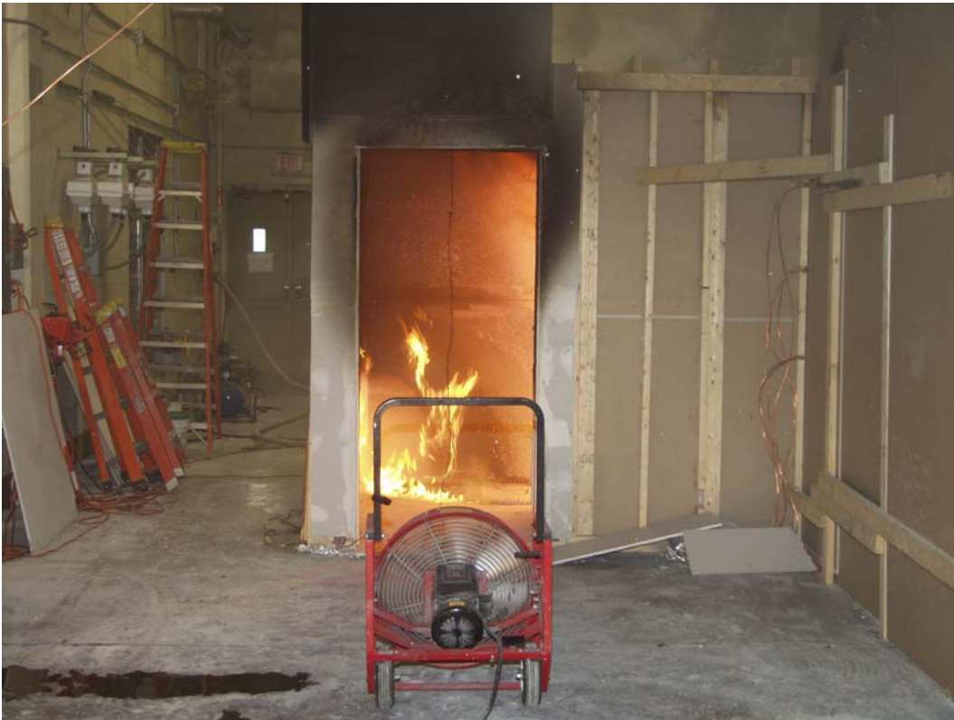
Figure 24 – Exterior View of Doorway to Corridor After the Start of Forced Ventilation (470 s)
