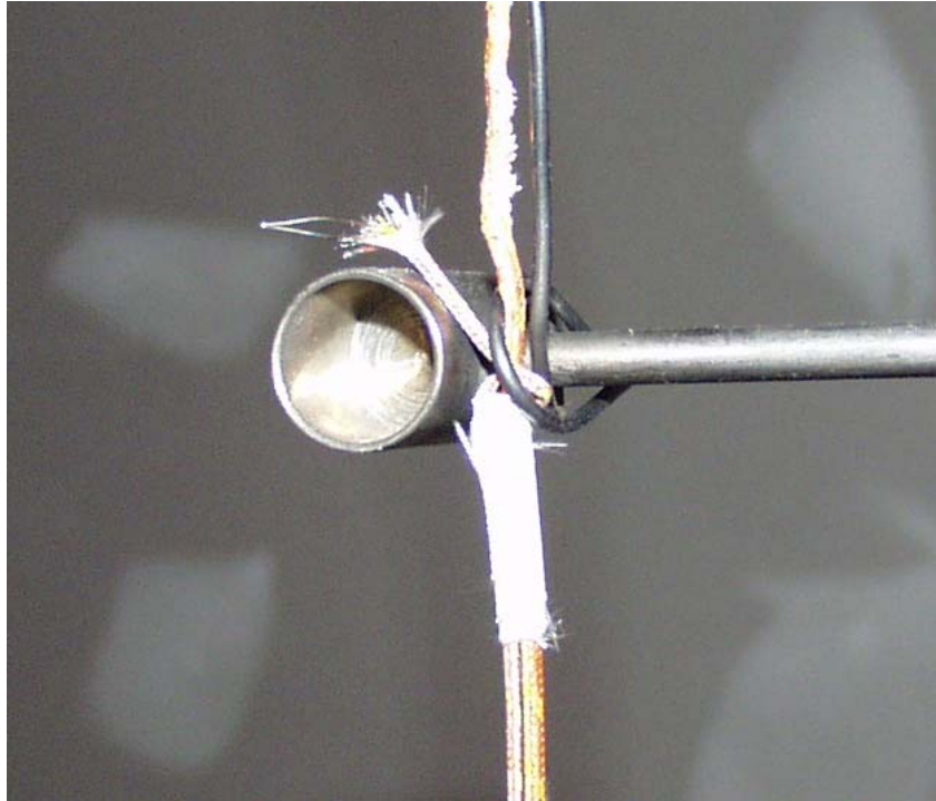
Figure 10 - Bidirectional Probe and Thermocouple Combination
