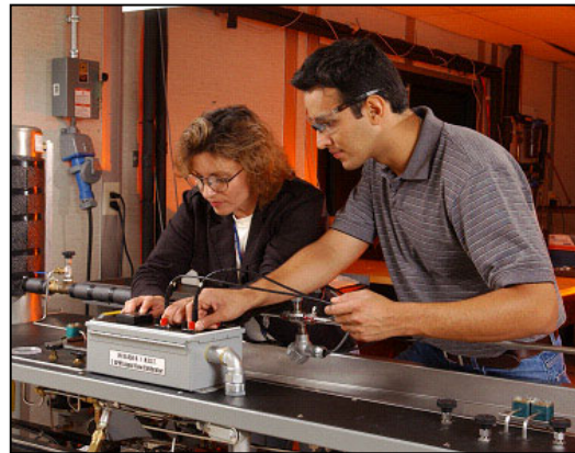
A dual rotor turbine meter is installed in the test section of the 2 L Hydrocarbon Liquid Flow Standard.
