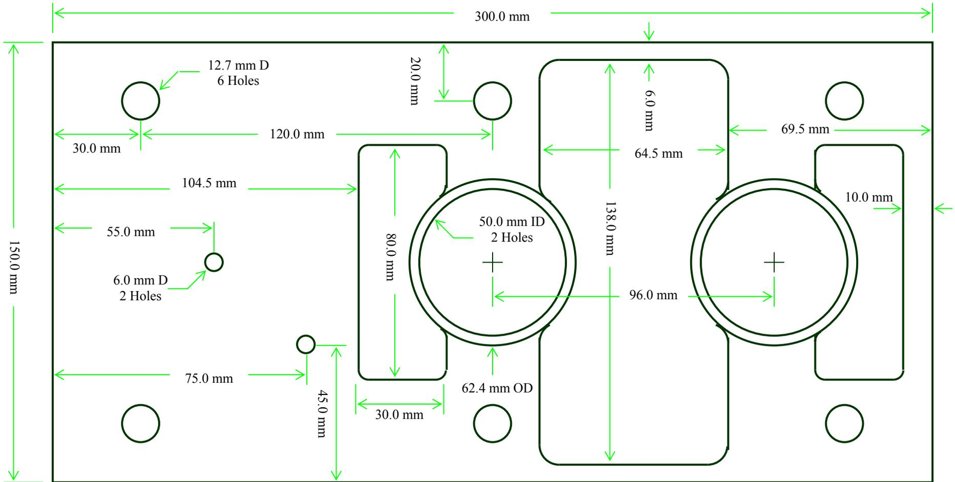
**Fig. 7 CAD Drawing of the Machine Part Specimen**
