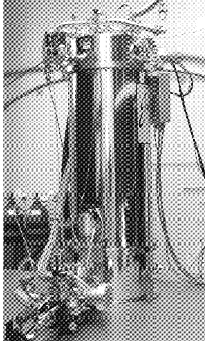
Figure 13. The Optical Technology Division’s second generation High-Accuracy Cryogenic Radiometer (HACR 2). HACR measures the absolute power of a laser beam used to calibrate silicon trap transfer standard detectors by comparing thermalized optical power to thermalized electrical power.
