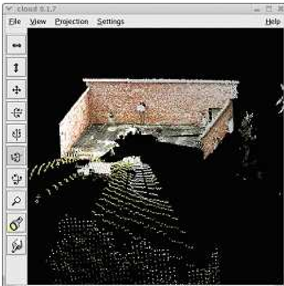
Figure 2 Data from a scan of orthogonal walls using the Riegl ladar.
