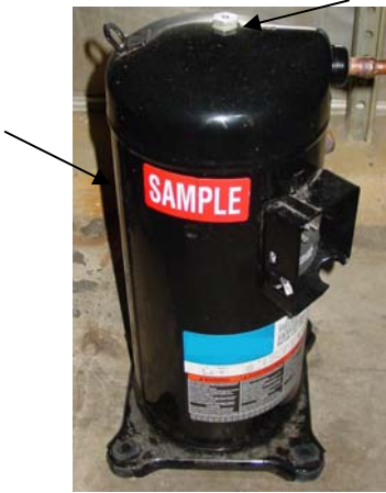
Figure 2.3.1: Hermetic, scroll compressor (the arrows on the picture indicate the position of the vibration sensor mounts)
