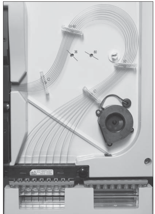
Sixteen capillaries enable high DNA throughput, allowing more samples to be simultaneously analyzed. © 2002 Robert Rathe
