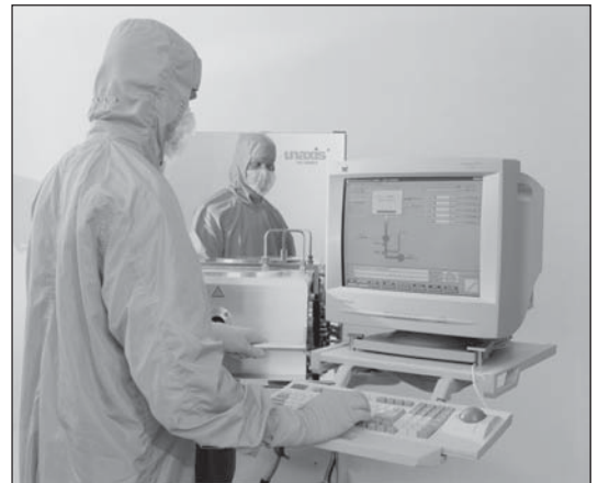
Unaxis 790 plasma etching and deposition system. [Property of Unaxis Wafer Processing, reprinted with permission]
