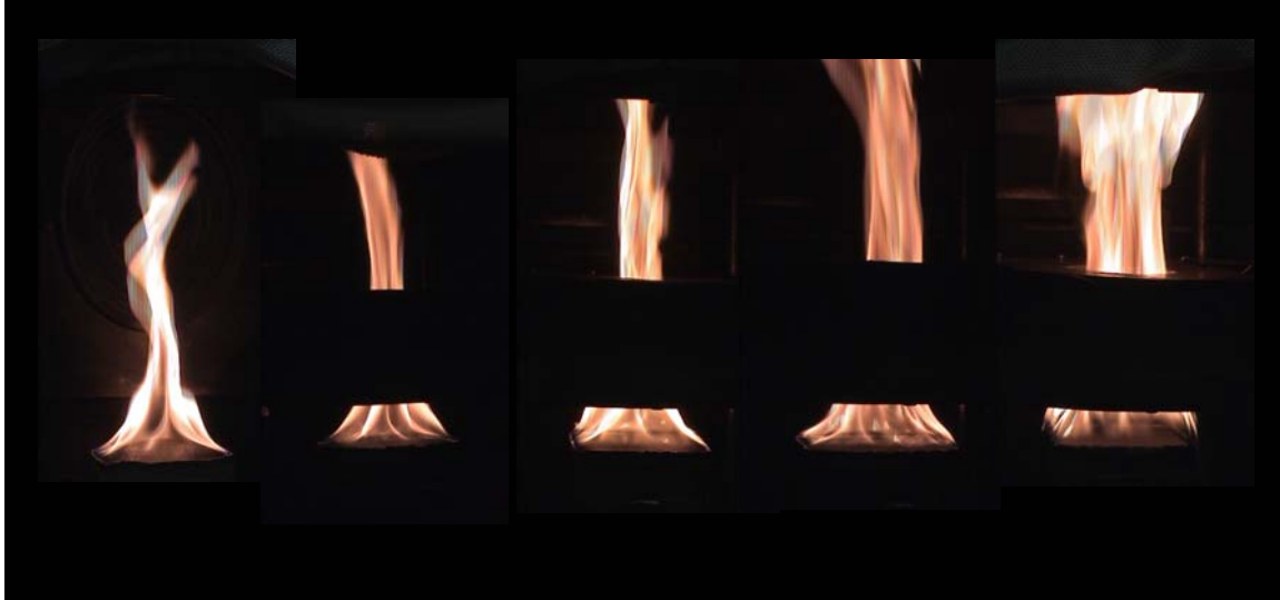
Figure 5 – Experimental flame images of PMMA samples burning in the horizontal configuration for (0, 5, 10, 25, and 75) kW/m 2 .
