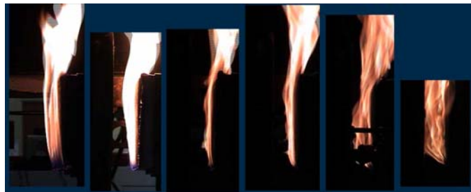
Figure 6 - Experimental flame images of PMMA samples burning in the vertical configuration for (0, 5, 10, 25, 50, and 75) kW/m 2 .
