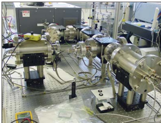
Figure 1. Measurement system for excimer laser power and energy calibrations at 157 nm.
