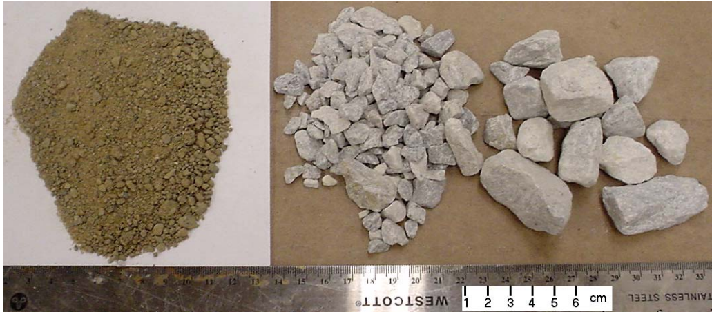
Figure 1: The aggregates used in the Cleveland test: Sand and gravel particles. As shown to the right, the aggregate size can be larger than 25 mm due to elongated shape.
