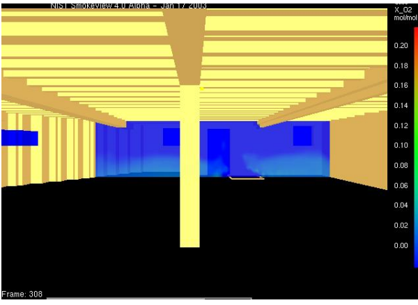
Figure 78. Oxygen Concentrations for an Initial 1000 kW Fire Source. Fire At Time = 1270 s. Fire Door is Open and Closing Mechanism Disabled.
