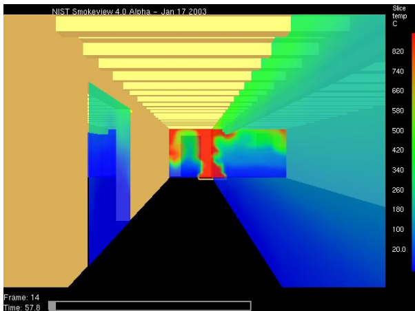
Figure 81. Temperature Profiles for an Initial 2000 kW Fire Source. Fire At Time = 58 s. Fire Door Open and Closing Mechanism Disabled.
