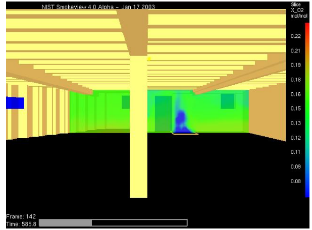
Figure 62. Oxygen Concentrations for an Initial 500 kW Fire Source. Fire At Time = 566 s. Fire Door Open and Closing Mechanism Disabled.
