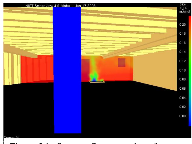
Figure 26. Oxygen Concentrations for an Initial 500 kW Fire Source. Fire At Time = 126 s. Fire Door Closed at 126 s.
