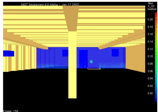
Figure 90. Oxygen Concentrations for an Initial 2000 kW Fire Source. Fire At Time = 644 s. Fire Door is Open and Closing Mechanism Disabled.
