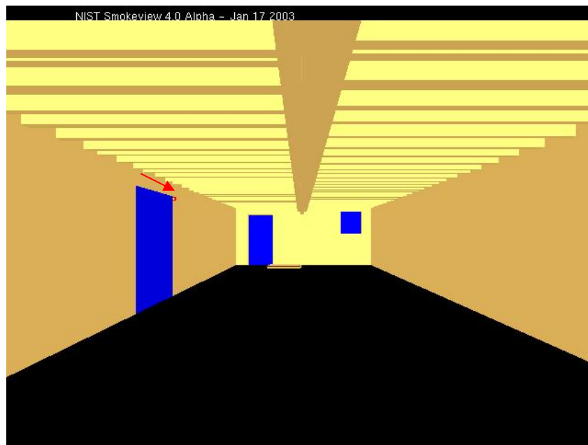
Figure 9. View Generated by Model Simulation Looking from Front of Unit 20 Towards Rear Door. Fire Door Opening Located in Wall on Left. Note Red Dot at Upper Right Corner of Fire Door Opening. Red Dot Indicates Position of Fire Door Thermocouple (next to location of fusible link).
