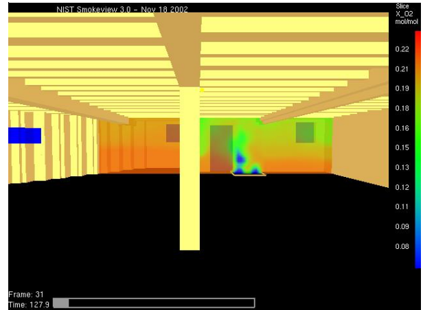
Figure 58. Oxygen Concentrations for an Initial 500 kW Fire Source. Fire At Time = 128 s. Fire Door is Open and Closing Mechanism Disabled.
