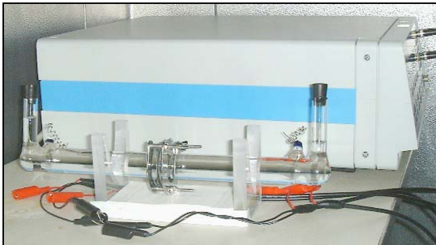
Figure 13. Setup for the bulk conductivity measurement (impedance spectrometer)
