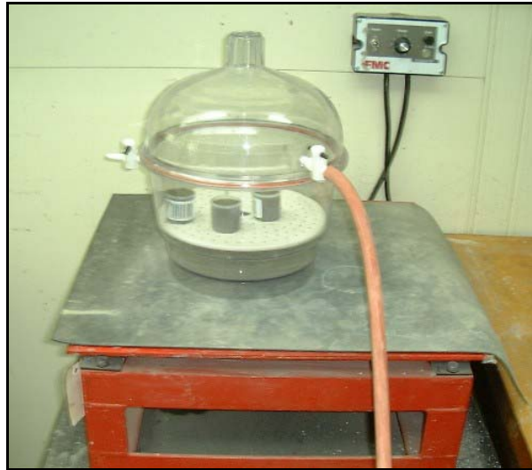
Figure 2. House vacuum container and vibrator used in paste preparation
