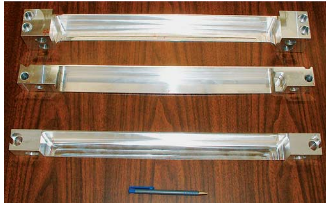
Figure 1: Aluminum parts machined to test shape changes caused by relaxation of residual stresses.
