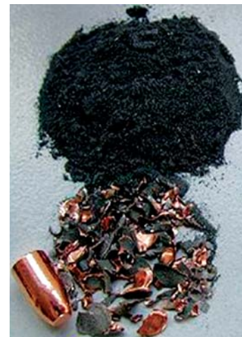
Figure 1: Frangible 9 mm bullet and remains after impact.
