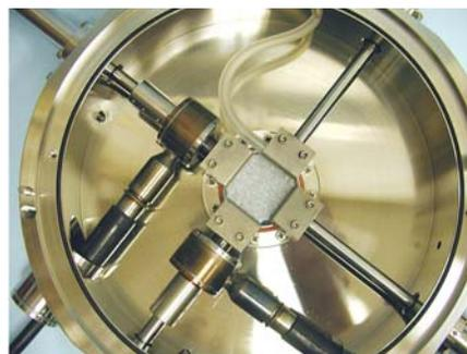
*Figure 1: The copper-colored load cells measure the applied force in this biaxial bioreactor. The sample is held in the center of the fixture and can be imaged from below to measure strain. The sample is bathed in nutrients (not shown), and the nutrient is also pumped across the surface of the scaffold through the grips.*
