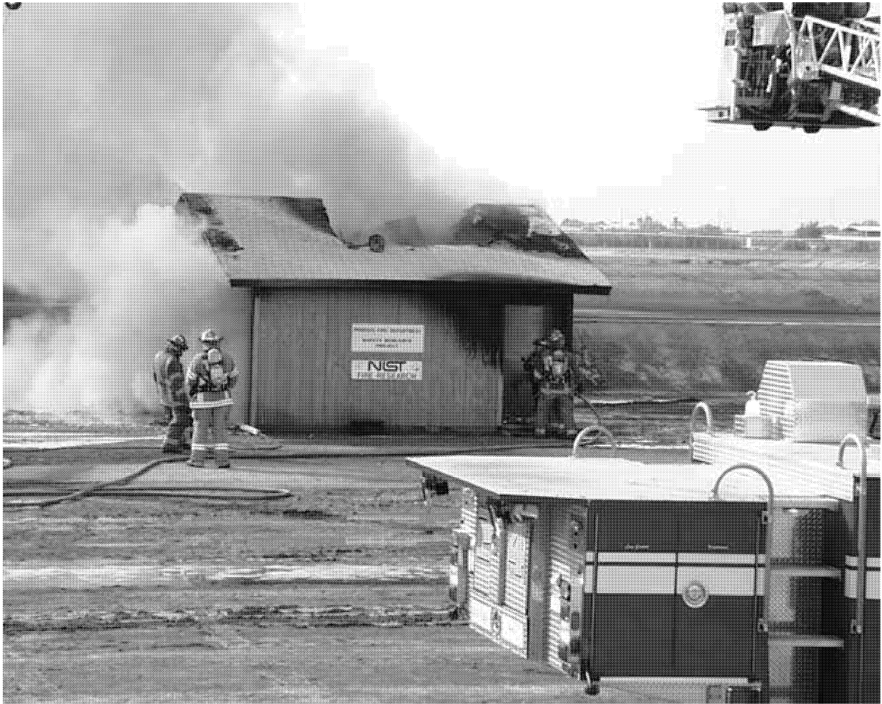
Figure 24. Photograph of test structure at 1140 s after ignition when suppression has been completed.
