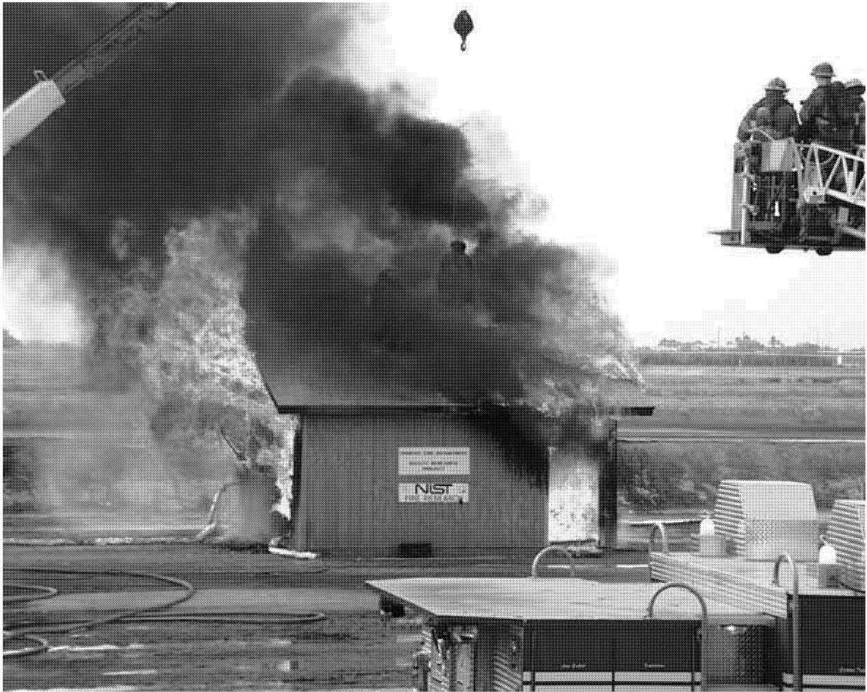
Figure 21. Photograph of test structure at 900 s after ignition when front door has burned away.
