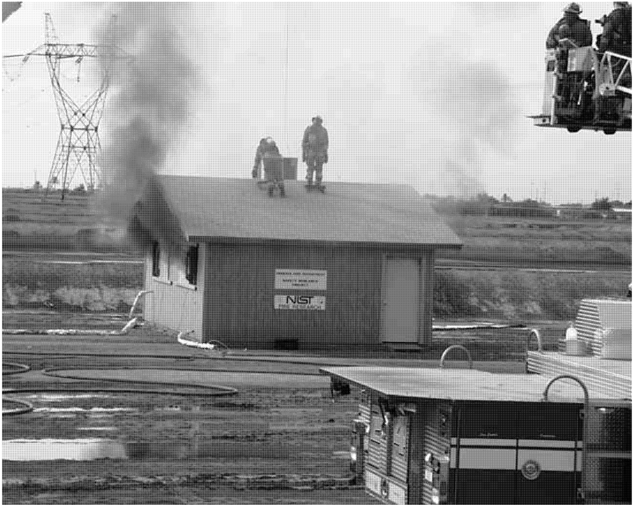
Figure 16. Photograph of test structure at 120 s after ignition.
