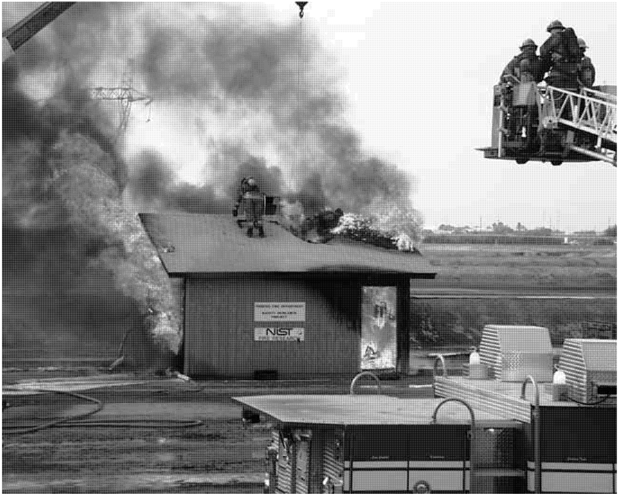
Figure 23. Photograph of test structure at 1010 s after ignition as collapse is starting.
