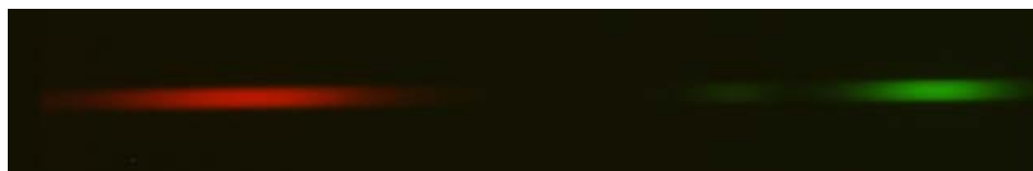
Fig. 2. Micellar gradient focusing and separation of two zwitterionic fluorescent dyes, rhodamine B (red) and rhodamine 110 (green). For scale, the image is 2 mm long.
