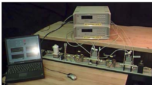
The transfer standard with its laptop data acquisition computer.
