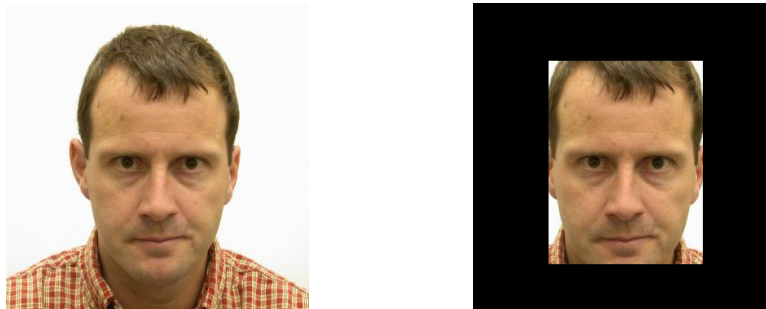
Figure 13: An image representative of the kind used in FRVT 2002, and a cropped version used to estimate the on-face compression ratio.
