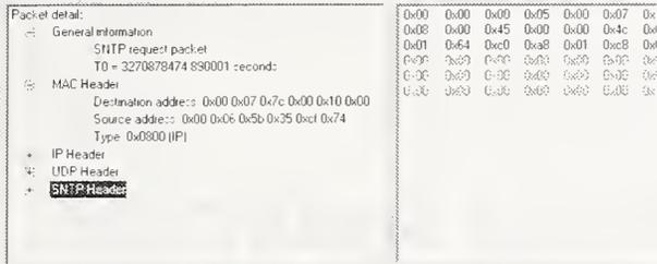
**Figure 7, visualization of a time synchronization packet**
