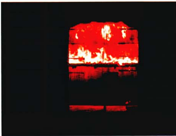
Figure 4. Cushion fire prior to flashover
