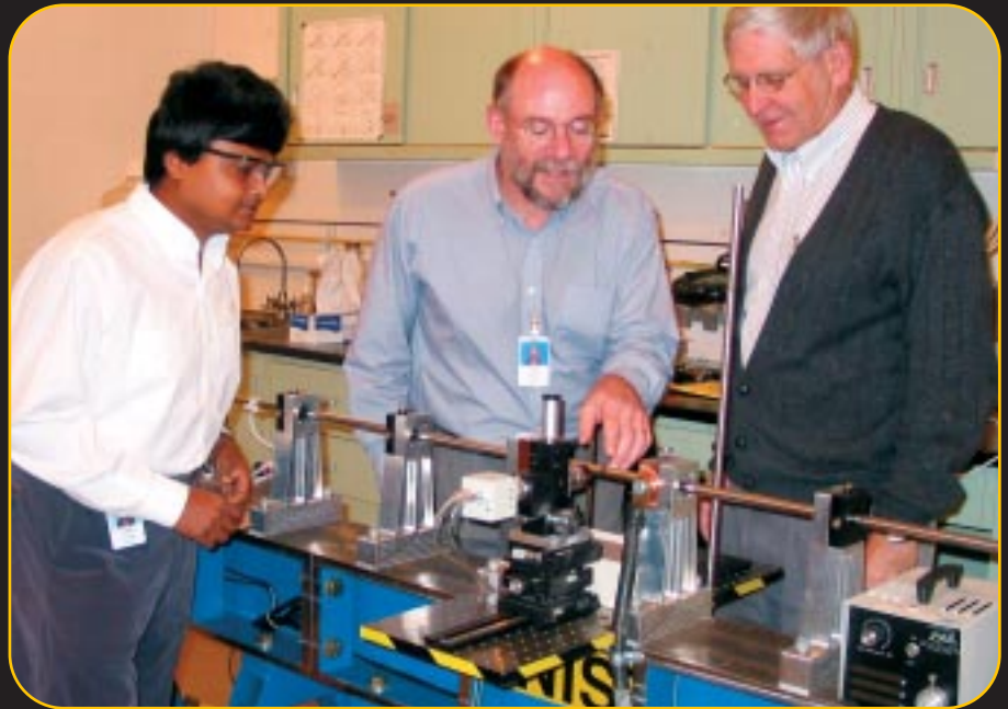
Tim Burns (center) discusses high strain rate materials testing with NIST collaborators Dick Rhorer (right) and Debasis Basak. The Kolsky Bar facility is being used to develop data for the development and validation of accurate simulation models.
