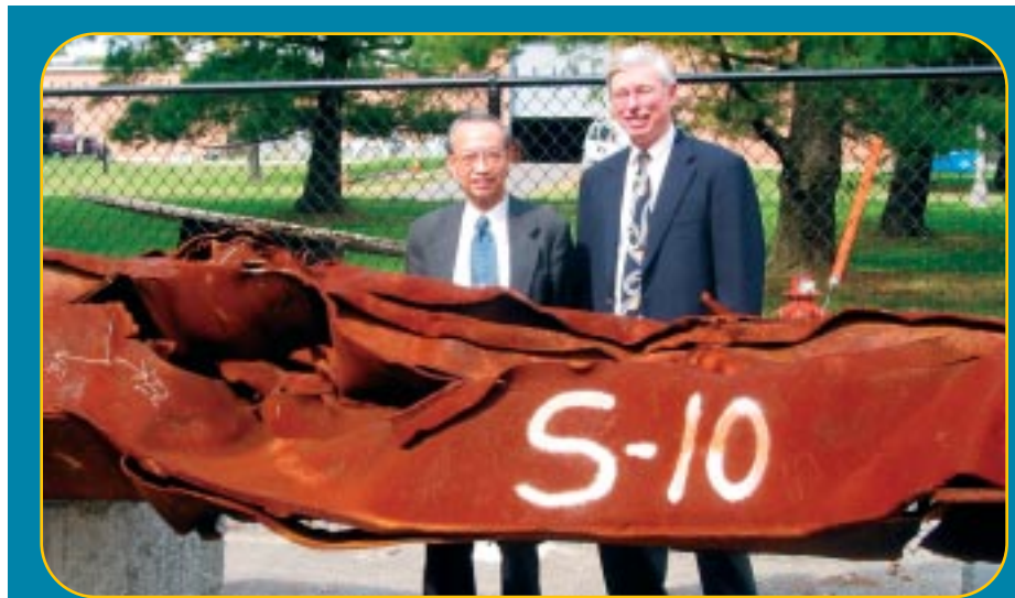
Jeffrey Fong and Jim Filliben, members of a NIST investigation team for determining the probable causes of the collapse of the World Trade Center (WTC) twin towers, pose behind part of a damaged three-column panel that used to be Panel #224 of the WTC North Tower in the middle of its east face between the 92nd and 95th floors. The panel, re-designated by NIST as S-10, currently sits at the NIST Gaithersburg site as part of a large number of damaged steels that were salvaged from Ground Zero and shipped to NIST following the September 11, 2001, disaster.
