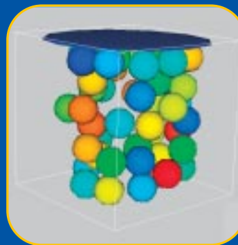
Visualization of a model rheometer (a device for measuring particle flow properties) under study using a quaternion-based dissipative particle dynamics code developed in collaboration with the NIST Building and Fire Research Laboratory.
