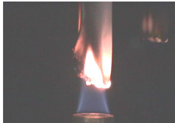
Figure 1. Standard 50 W UL94 test flame applied to specimen in vertical burn test.
