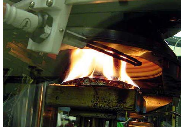
Figure 2. Cone Calorimeter test at 50 kW/m 2 .
