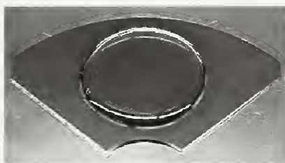
Figure 2: Confined lubricant solution on a hard disk.
