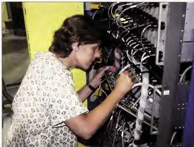
Fig. 3. Doris Kendig (NCNR) adjusts motor drivers on the new motor control system.
