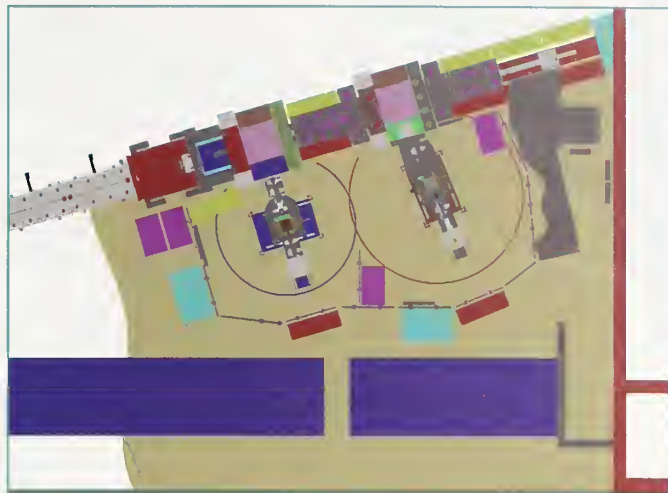
AND/R (right) and NG-1 Reflectometer floor plan. The large circles indicate the travel of the detector arm in its fully extended position. Blue, purple and red rectangles are the control desks, electronic racks and beamstops respectively. The instruments will be separated by both a fixed rail and a tensile barrier (not shown).
