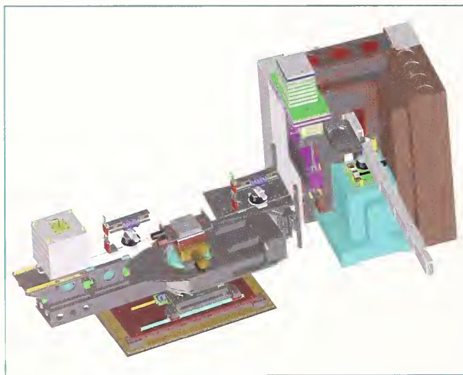
The Advanced Neutron Diffractometer Reflectometer, shown in polarized beam mode with the "pencil" detector enclosed within the box at left. (For clarity, some shielding is not shown.)
