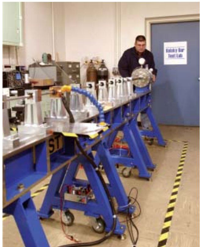
Figure 1b: Photograph of NIST's Kolsky Bar facility.
