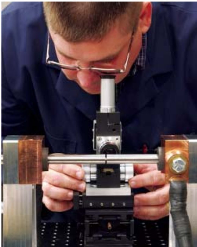
Figure 2: The current for heating is introduced through copper blocks and graphite bearings to the incident and transmitted bars, and then through the sample seen in the middle. The sample temperature is monitored by the pyrometer being focused on it.
