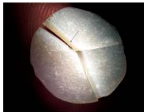
Figure 1: ACP composite disk (16 mm D x 1 mm H) after biaxial flexure loading. Note the polyethylene fibers bridging the crack near the center of the fractured disk.
