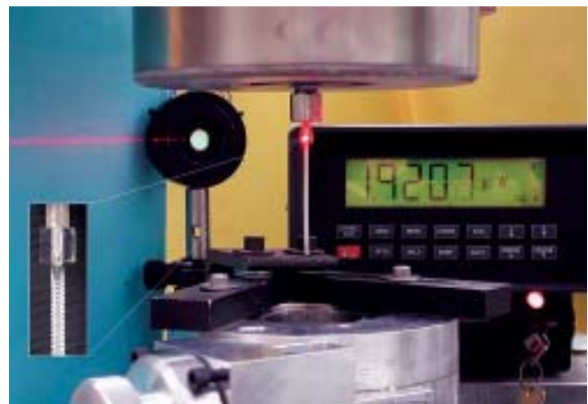
Figure 2: Frustrated Total Internal Reflection optics is installed near the die exit on a capillary rheometer. The amplitude of the reflected light allows a determination of the coating thickness.
