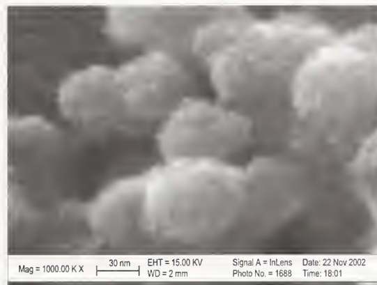
Figure 1: Scanning electron microscope image of the surface of a copper electrodeposit at a magnification of 1 million.
