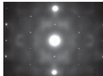
Figure 4: High-index zone axis electron diffraction pattern from the pyrochlore \text{Bi}_{1.5}\text{Zn}_{0.92}\text{Nb}_{1.5}\text{O}_{6.92} reveals well-structured diffuse scattering likely associated with local ordering of Bi and Zn.
